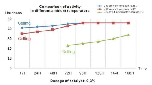
Maintaining high catalytic activity in a low temperature (0-10 °C) environment in winter. It can significantly increase the winter construction period by providing sufficient strength for the subsequent process construction on the second day of paving construction.
